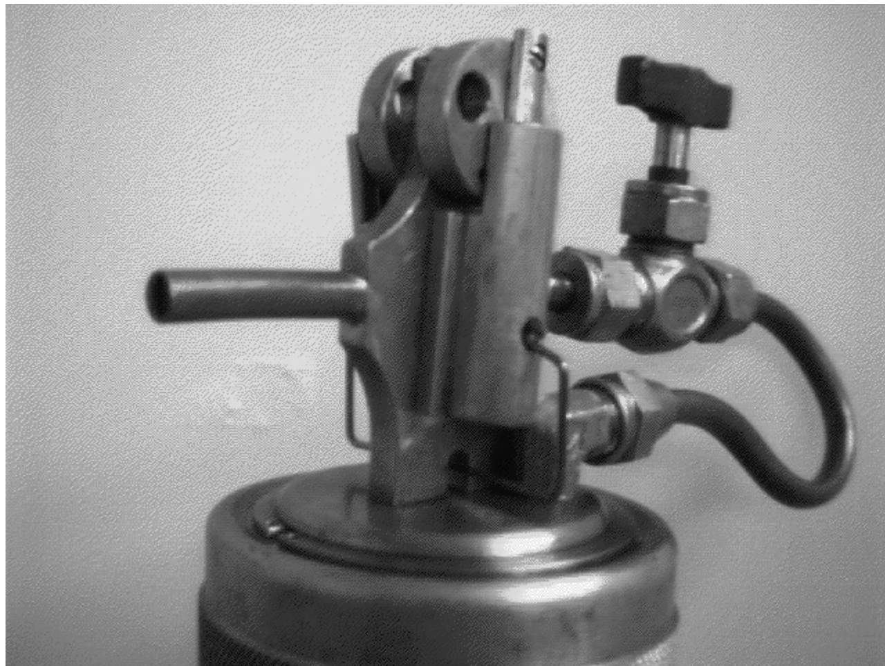
FIGURE 2. CLOSE-UP VIEW OF ASSEMBLED LIQUID NITROGEN FUELED ENGINE.
