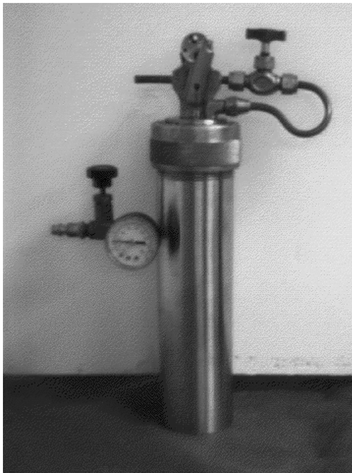
FIGURE 1. VIEW OF THE ASSEMBLED LIQUID NITROGEN FUELED ENGINE, INCLUDING LIQUID NITROGEN RESERVOIR.
